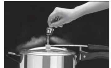
Once steam is coming out of the steam vent steadily, place the pressure regulator on the steam vent and press down firmly. Keep fingers on top of the pressure regulator and away from the steam when placing the pressure regulator on the steam vent. A click indicates that the pressure regulator is in position. In about 2 minutes, the cooker should come to full operating pressure.
